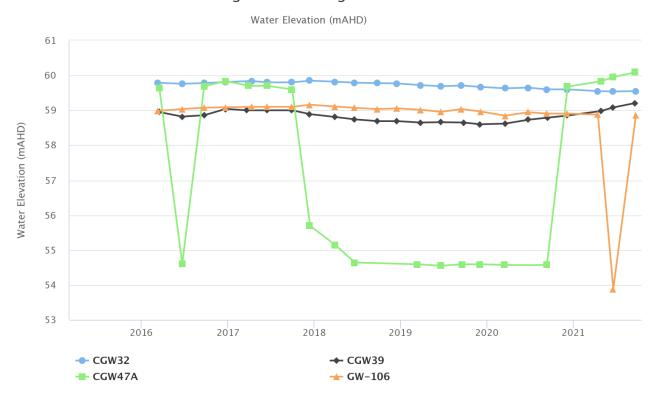
Figure 44 - Carrington West Wing Flood Plain Water Elevation Trend - Q3 2021
