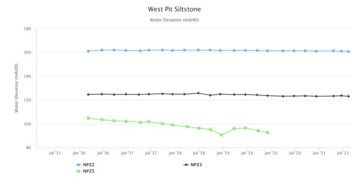
Figure 65 - West Pit Siltstone Water Elevation Trend - Q3 2021
