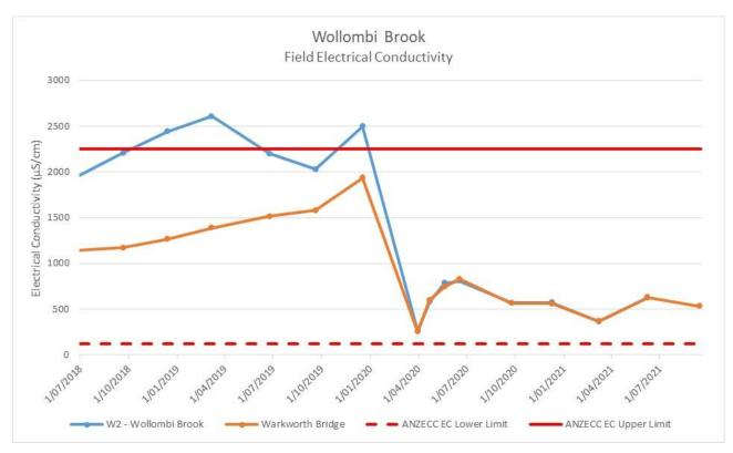
Figure 17 - Wollombi Brook Electrical Conductivity - September 2021
