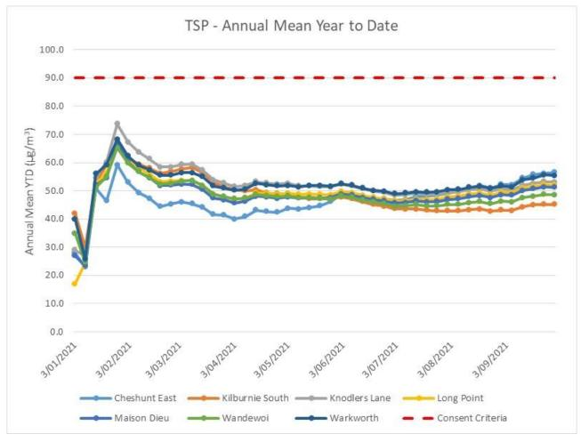
Figure 10 - Year to Date Average Total Suspended Particulates as at end of the Reporting Period
