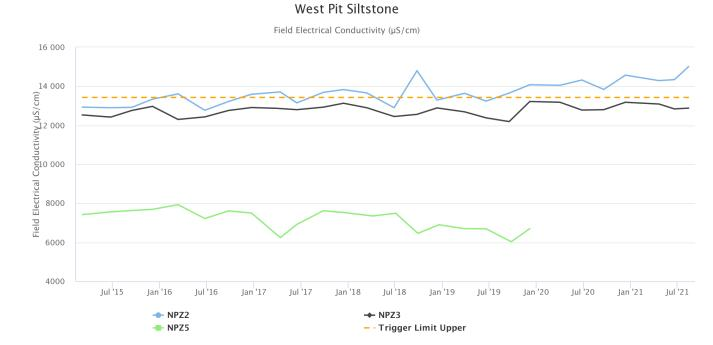
Figure 63 - West Pit Siltstone Electrical Conductivity Trend - Q3 2021
