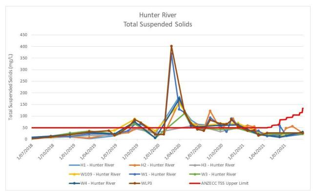
Figure 22 - Hunter River Total Suspended Solids - September 2021
